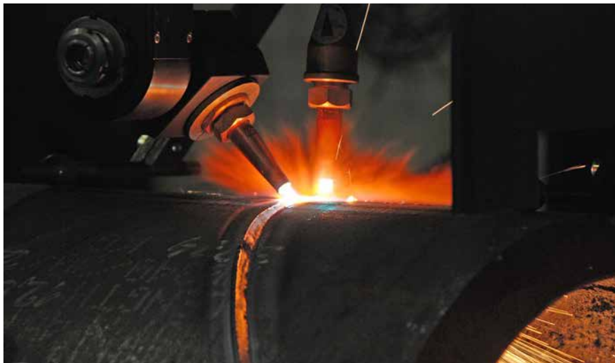
Steel cutting with pre-heater
