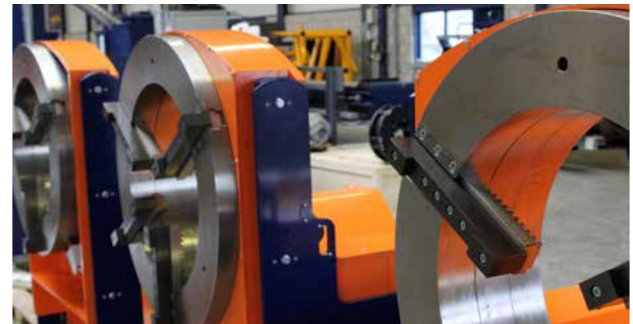
Left small diameter with outside clamping. Right inside clamping for larger diameters.
