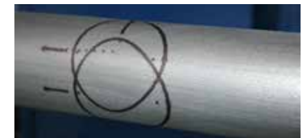
Footprint marking double saddle Ink-jet
