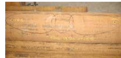
Footprint marking triple saddle
